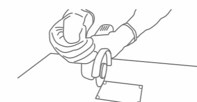
To get internal and L-shaped corners & to reduce the risk of breakage, round off the vertex of the internal corner using bits with a radius of at least 5mm. Then cut with diamond discs, be cautious to stop moving the cutting tool forward. To drill and cut using diamond discs, follow the instructions provided above.
